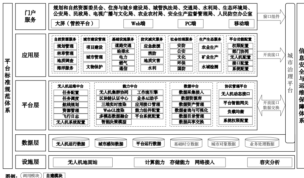
Fig. 1 Overall architecture design of UAV management platform
